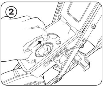
Insert the seed plate into the SRS hopper by placing it over the centre of the mounting and turning the plate clockwise to lock it into position.
