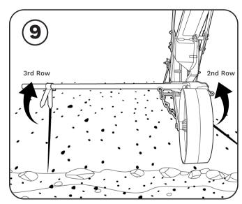
Stop at the end of the first run and place the marker back in its holder in the vertical position. The marker will have left a trail to be followed for the next seeding row (2nd Row). Now place the marker on the opposite side (on your left) and push the seeder along the track made by the marker on your first run (2nd Row).
