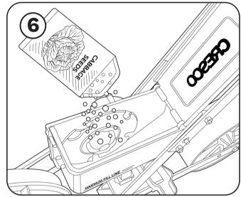
Empty the seeds into the hopper but make sure you do not exceed the maximum fill line. Overfilling can result in over application which will damage your yield.
