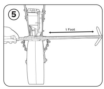
Adjust the row marker to the correct distance as shown
